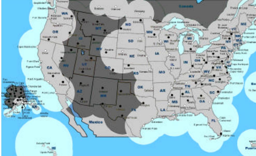
**Figure 6.10** GPS Differential Beacon Coverage in North America in 1999. Beacons along the coast areas are operated by the U.S. Coast Guard. Beacons along navigable rivers have belong to the U.S. Army Corps of Engineers. Many inland states have also constructed beacons.
