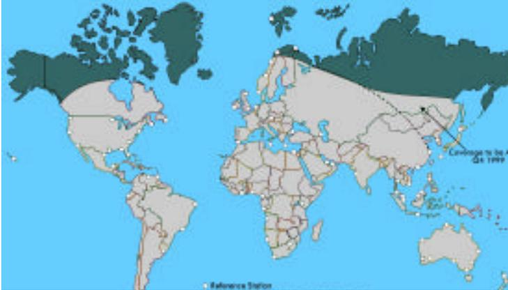
**Figure 6.9** World Differential GPS Coverage by privately owned satellites. Omnistar provides differential GPS data from ground stations via satellite. A special receiver is needed to download the differential data from the private satellite. This data is then compared to that received by the GPS receiver.
