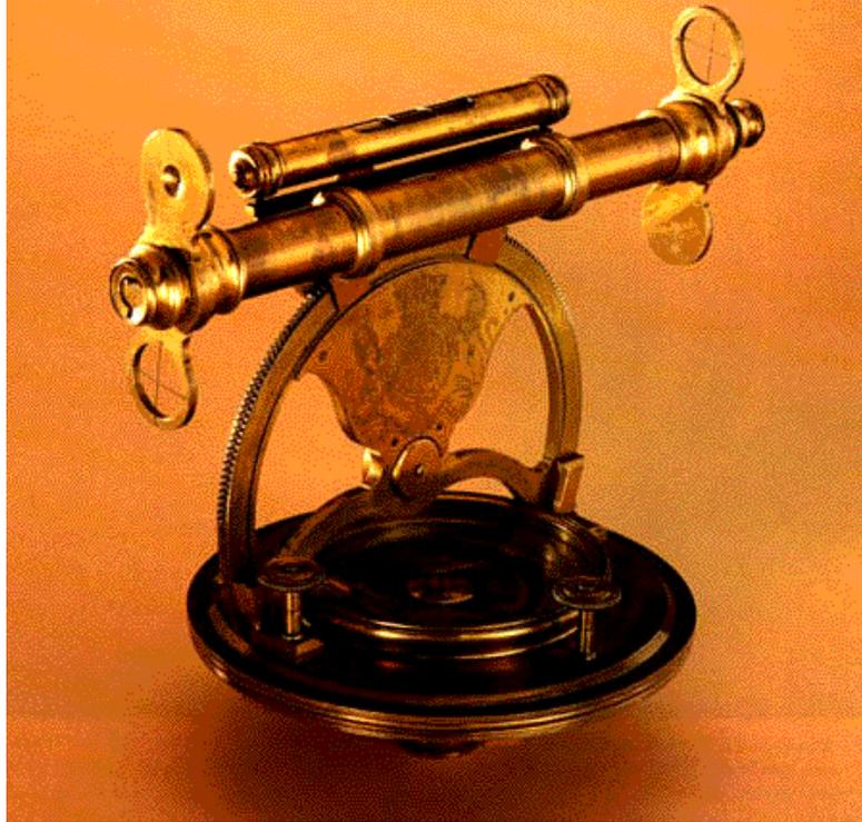
**Figure 6.13** The Duke of Cumberland's theodolite. Benjamin Cole, a prominent London instrument maker, made this theodolite for the Duke of Cumberland, George III's uncle, in the 1740s or 1750s. A theodolite is a surveying instrument that measures both horizontal and vertical angles. A new invention in the eighteenth century, the theodolite was not in fact widely used until the nineteenth. Science Museum/Science & Society Picture Library.
